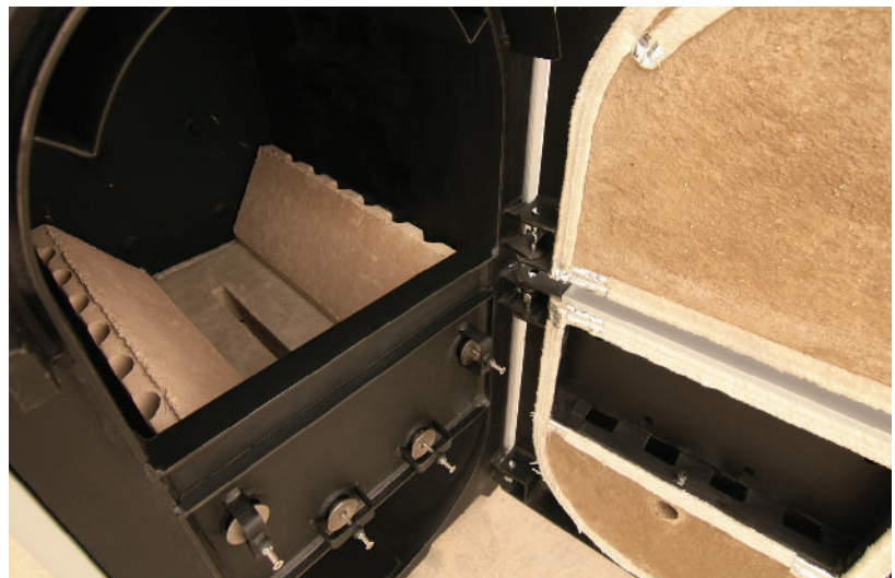
Pre-Heating canals interior view
