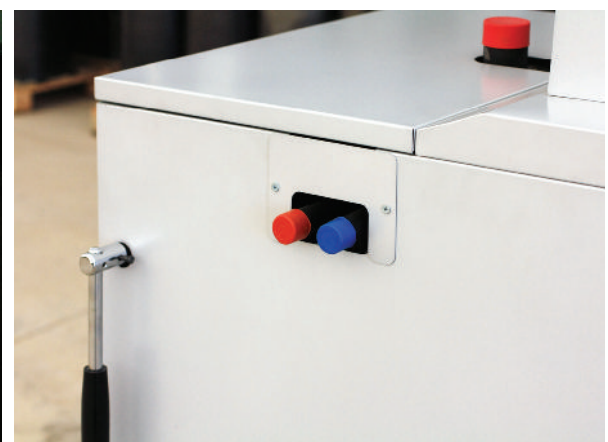
Interchangable copper Emergency flush system
