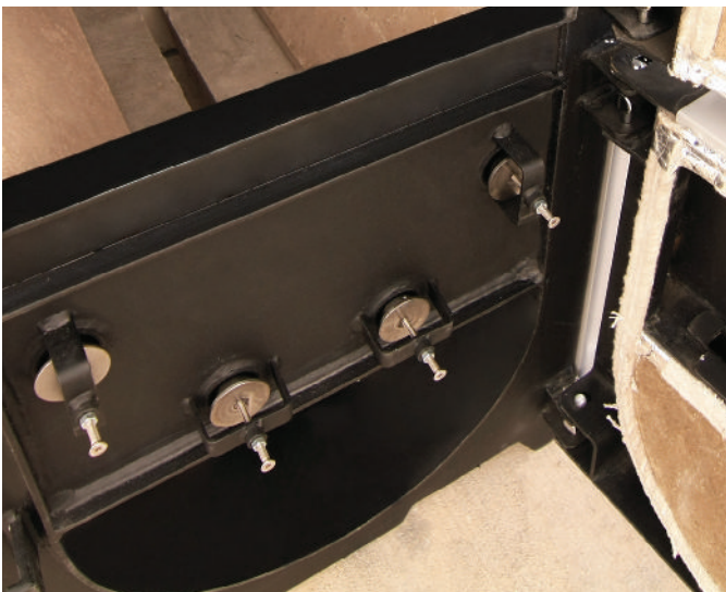
Independently adjustable Primary and secondary air inlets
