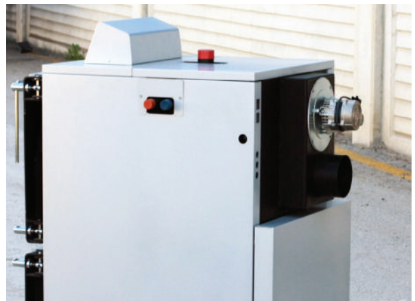
Induced draft fan keeps the system in constant vacuum eliminating the possibility of a smoke leakage to the ambient.
