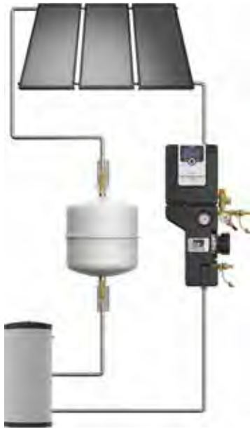
Mounting example with collector field and buffer tank
