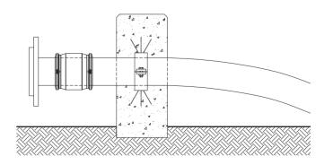
Figure 57.3: Anchoring the pipe end
