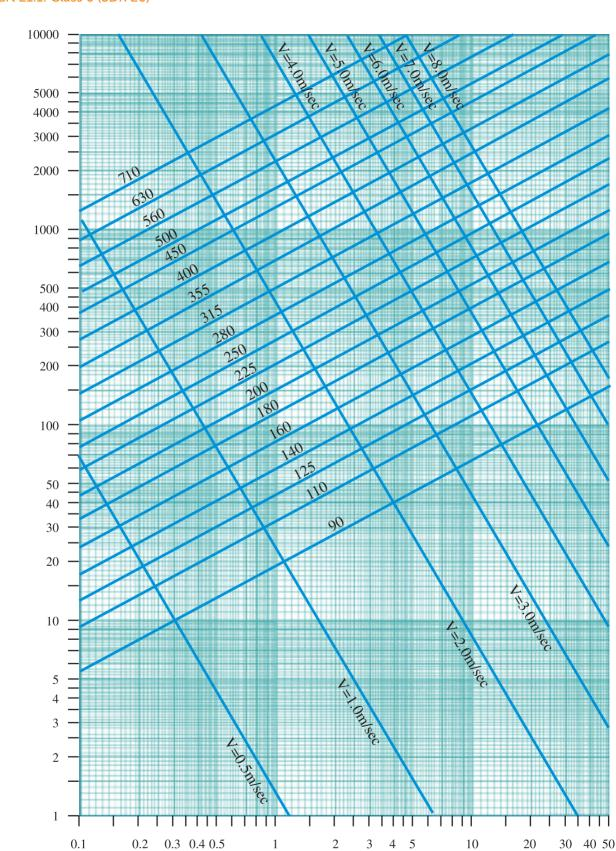
Head Loss [meters] for 100 meters Pexgol pipe
